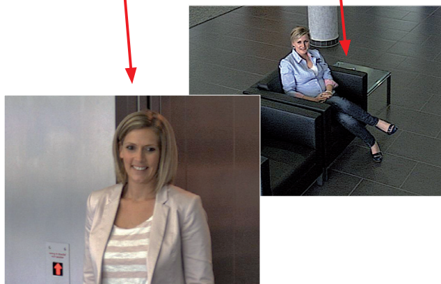
Original image: Telephoto lens (left) and wide angle lens (right) – simultaneously in one image
