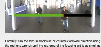
possible. Remove the lens wrench every time you changed the lens focus. Once the focus is adjusted properly, deactivate the focusing aid again (Focusing Aid quick control, Disabled value).
